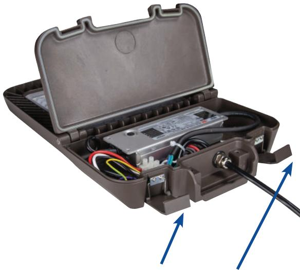
The TAL Area Light features clips on the rear of the fixture to close the electrical compartment. These clips open and close without the need for tools, making maintenance and repairs in the field simple.
