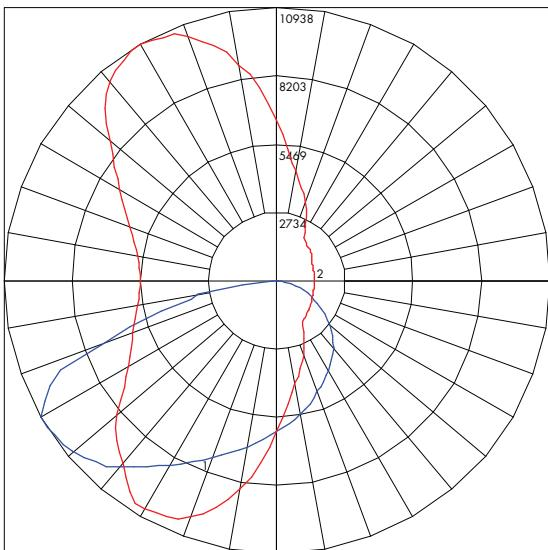
Maximum Candela = 10937.78 Located At Horizontal Angle = 120, Vertical Angle = 57.5
