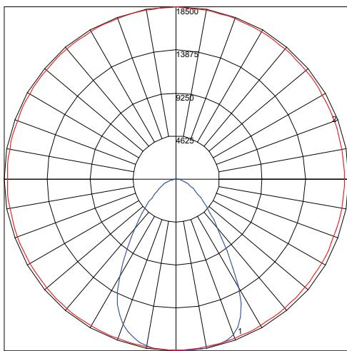
Maximum Candela = 18499.5 Located At Horizontal Angle = 270, Vertical Angle = 5
