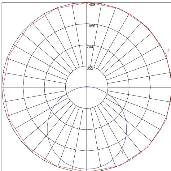
Maximum Candela = 1407.6 Located At Horizontal Angle = 0, Vertical Angle = 0
