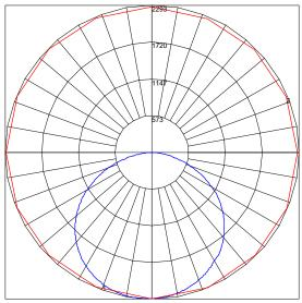
$\label{eq:maximum Candela = 2293.1 Located At Horizontal Angle = 270, Vertical Angle = 3.5 #1 - Vertical Plane Through Horizontal Angles (270 - 90) [Through Max. Cd.] #2 - Horizontal Cone Through Vertical Angle (3.5) [Through Max. Cd.]$
