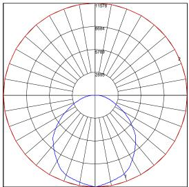
Maximum Candela = 11578 Located At Horizontal Angle = 0, Vertical Angle = 0 # 1 - Vertical Plane Through Horizontal Angles (0 - 180) (Through Max. Cd.) # 2 - Horizontal Cone Through Vertical Angle (0) (Through Max. Cd.)
