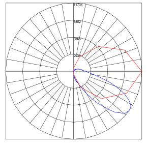
Maximum Candela = 11736 Located At Horizontal Angle = 00, Vertical Angle = 55 # 1 - Vertical Plane Through Horizontal Angles (0 - 180) (Through Max. Cd.) # 2 - Horizontal Cone Through Vertical Angle (55) (Through Max. Cd.)
