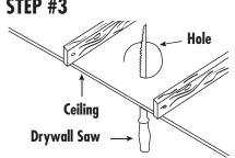
Carefully make a fixture installation hole in the ceiling using a drywall saw.
