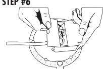
Replace wiring compartment door. Ensure it is closed securely. Make sure airtight gasket is positioned on back of trim.
