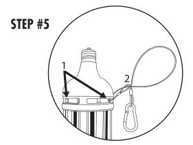
If lamp being installed is over 60w, attach provided tether cable to lamp. Locate either entry hole(1) on lamp shown in diagram and feed looped end of tether cable(2) through hole. You may need to crimp with pliers first. Once through, take end with grappling clip through loop as shown, tighten and secure clip to safe location.
