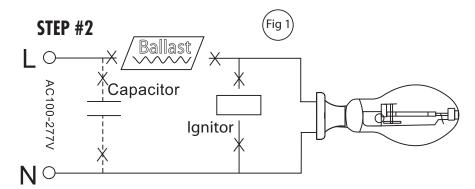
Remove old ballast or disconnect from existing lamp holder. Remove and dispose of ballast in correct manner (also disconnect any other components such as ignitors, starters, capacitors). Shown as Figure 1.
