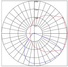
${\sf Maximum\ Candela=2085.871\ Located\ At\ Horizontal\ Angle=330,\ Vertical\ Angle=53}$
