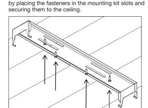
Step 2: Secure the mounting bracket using appropriate
