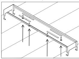
**Step 4:** Line up one end of the curved metal hooks with the hanging chains on one end of the QHB body.
