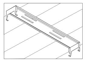
**Step 3:** Line up one end of the curved metal hooks with the slots on one end of the QHB body.
