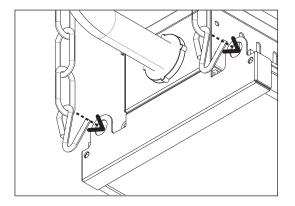
**Step 2:** Secure the mounting bracket using appropriate customer supplied anchor screws, toggle bolts or suitable fasteners (depending on structural conditions) by placing the fasteners in the mounting kit slots and securing them to the ceiling.
