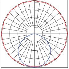
Maximum Candela = 10575.88 Located At Horizontal Angle = 90, Vertical Angle = 1 # 1 - Vertical Plane Through Horizontal Angles (90 - 270) [Through Max. Cd.]
