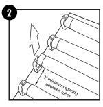
Remove fluorescent lamps. Dispose of fluorescent lamps per local requirements and codes for mercury disposal. Gain access to ballast by removing cover.
