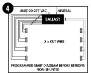
Wiring diagrams of PROGRAMMED START.
