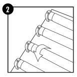
Verify that the tube being removed is compatible with the T8 lamp.Twist fluorescent tube until slots are visible.
