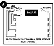
Revised wiring diagrams of PROGRAMMED START.
