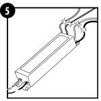
Cut all wires to ballast (close to ballast case). DO NOT REMOVE BALLAST! Keep ballast in place. Rewire according to Step 6.
