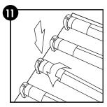
Install ballast cover. Install T8 lamps.
