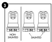
Check whether lamp holders (tombstones) are shunted, indicating Instant Start. If shunted, proceed to Step 7. Non-shunted tombstones indicate Programmed Start. If PS, proceed to Step 4 for wiring diagram.
