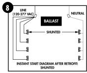
Revised wiring diagrams of INSTANT START. DO NOT REMOVE BALLAST! Keep ballast in place.
