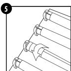
Twist T8 lamp to secure until resistance is met. Make sure light emitting side is facing out. Replace all lamps and diffuser.
