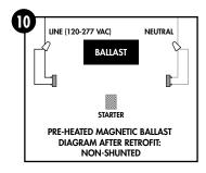
Revised wiring diagrams of PRE-HEATED MAGNETIC BALLAST. DO NOT REMOVE BALLAST! Keep ballast in place.
