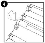
Line both ends of T8 lamp into slots.
