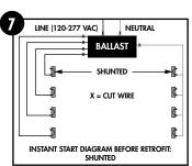
For INSTANT START: Cut wires indicated in diagram. Attach leads together with wire nuts, as shown in
