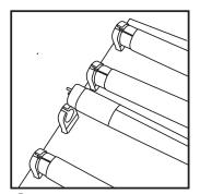
Line up both ends of T5 lamp into slots.
