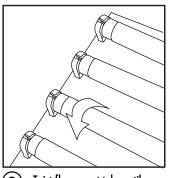
Twist fluorescent tube until slots are visible.
