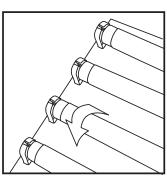
Twist T5 lamp to secure until resistance is met. Make sure light emitting side is facing out. Replace all lamps.
