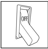
Switch OFF Power to the luminaire. If luminaire is equipped with a diffuser, remove at this time.
