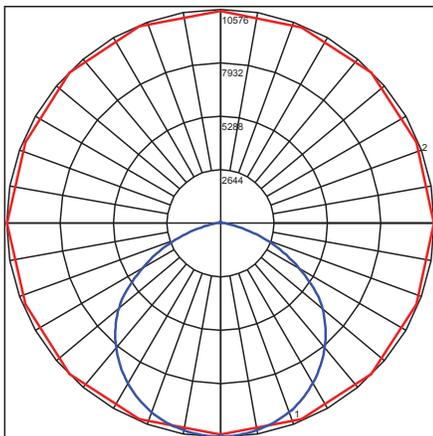
Maximum Candela = 10575.88 Located At Horizontal Angle = 90, Vertical Angle = 1
