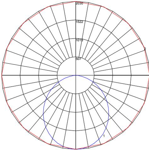
Maximum Candela = 1671.01 Located At Horizontal Angle = 10, Vertical Angle = 5
