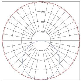
$\label{eq:maximum Candela} $$ Maximum Candela = 1808.2 \ Located At Horizontal Angle = 0, Vertical Angle = 0 $$ \# 1 - Vertical Plane Through Horizontal Angles (0 - 180) [Through Max. Cd.] $$ \# 2 - Horizontal Cone Through Vertical Angle (0) [Through Max. Cd.] $$$
